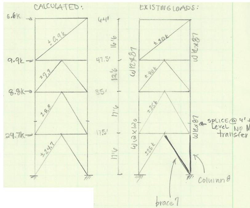
Figure 48: Elevation of braced frame 2, with verified members highlighted on right.
