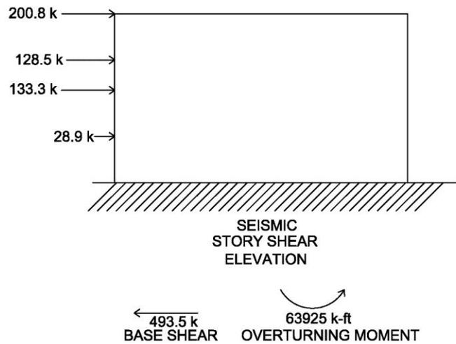
Figure 28 : Summary of forces due to seismic loads.
