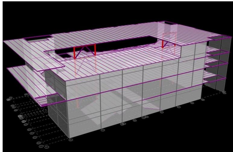
Figure 31: RAM lateral model from the Northeast corner of the building.
