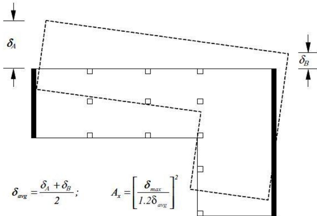
FIGURE 12.8-1 TORSIONAL AMPLIFICATION FACTOR,  $A_x$
