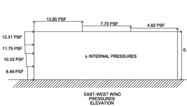
Figure 17: Summary of East-West wind pressures in elevation.
