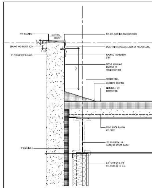
Figure 9 : Cross section of the roofing system.
