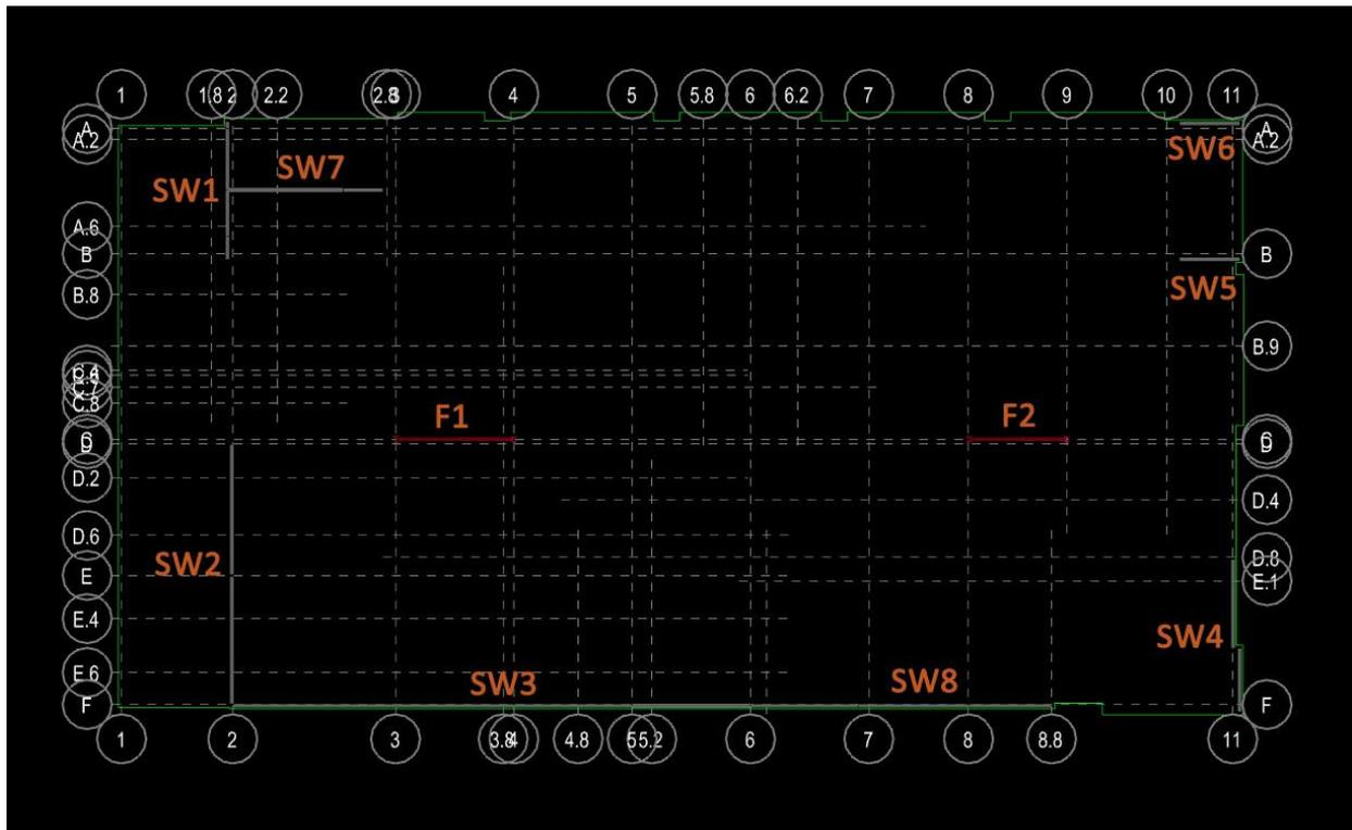
Figure 33: Floor plan displaying frame and shear wall designations.
