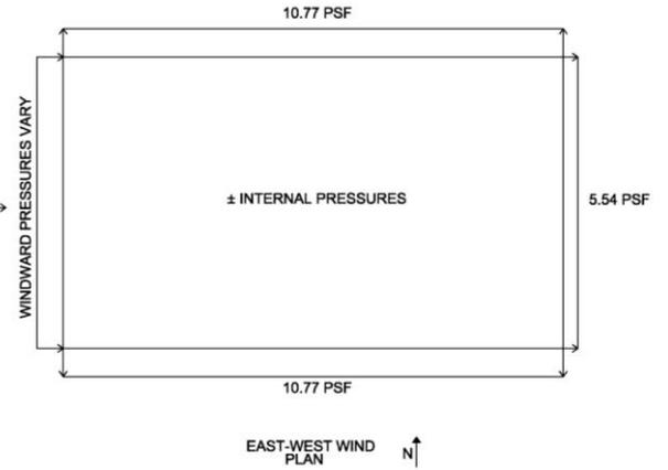
Figure 18: Summary of East-West wind pressures in plan.
