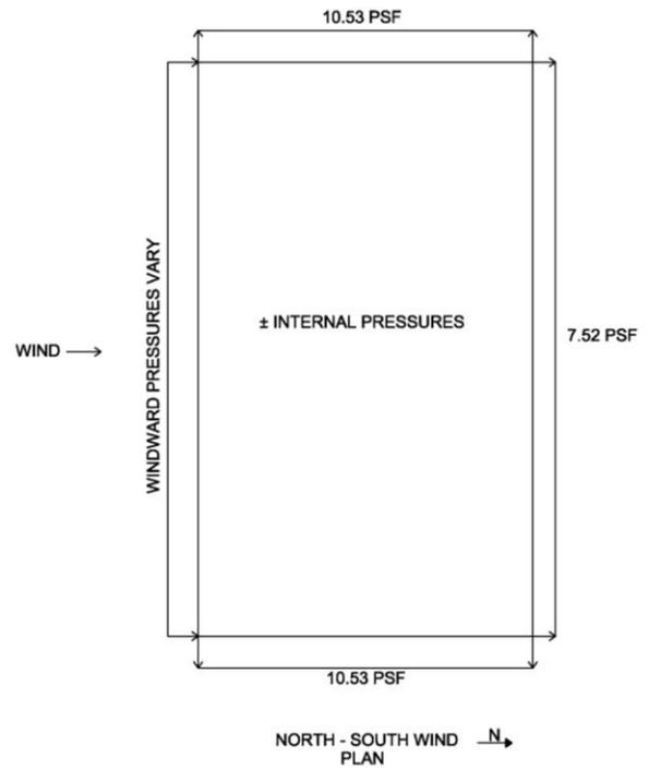
Figure 23: Summary of pressures in the North-South direction in plan.
