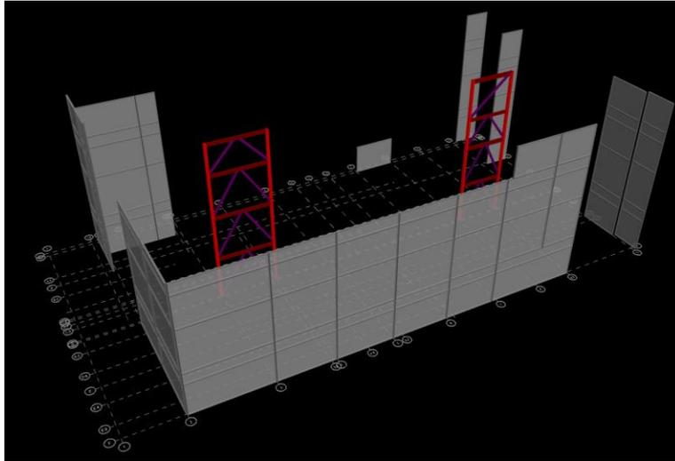
**Figure 32:** RAM model showing lateral system without diaphragms.
