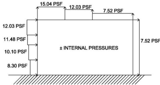
Figure 21: Summary of forces in the North-South direction in elevation.
