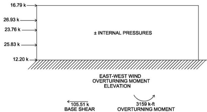
Figure 20 : Summary of final forces in East-West direction in elevation.
