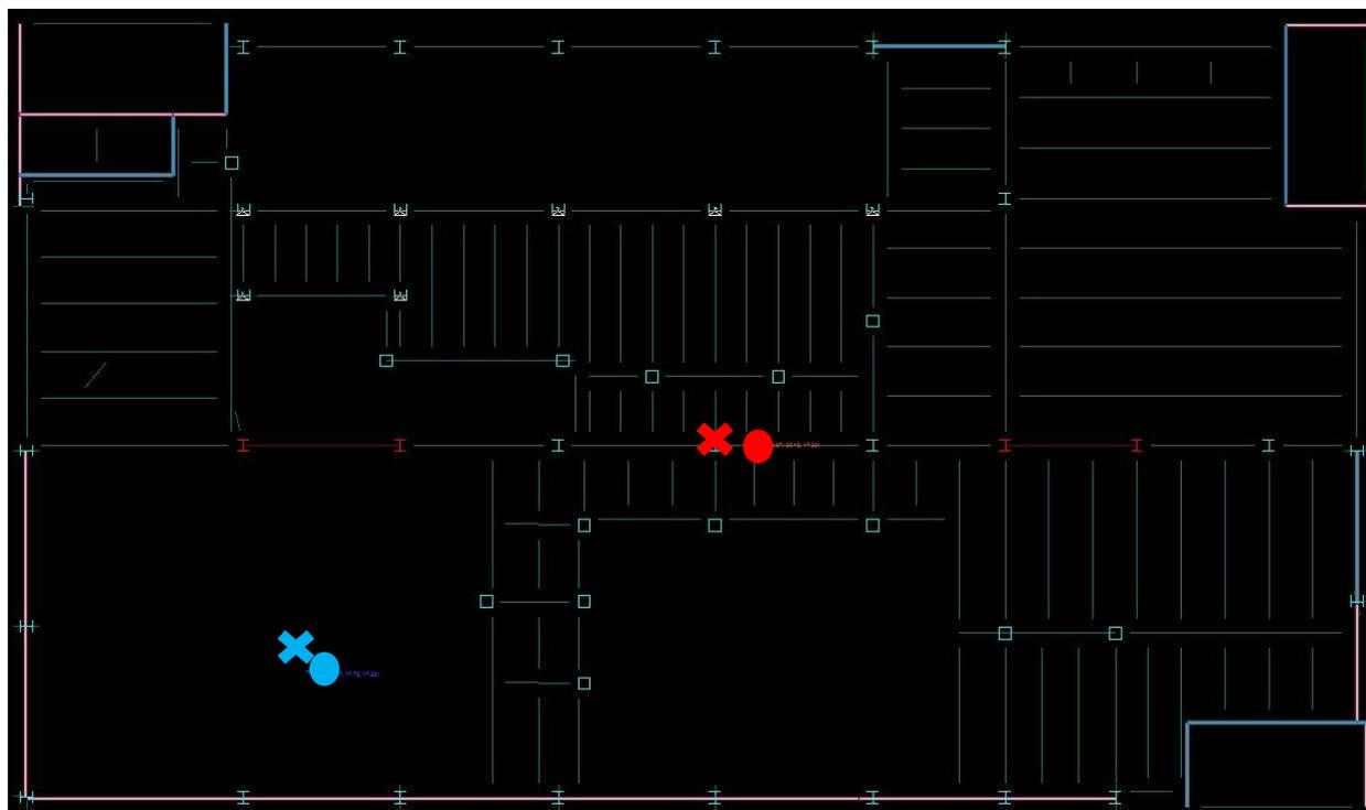
Figure 37: Second floor plan displaying center of rigidity (blue) and center of mass (red).
