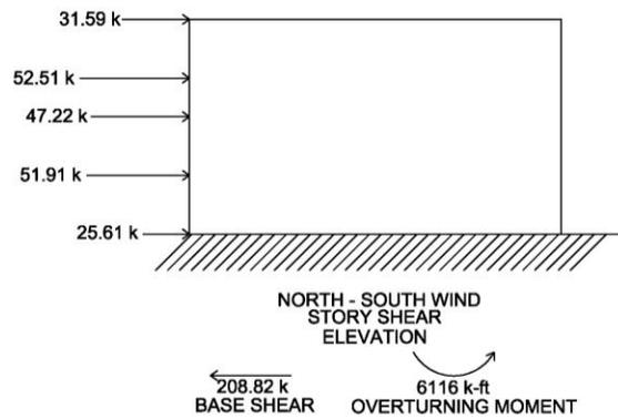
Figure 24 : Summary of final forces in North-South direction in elevation.
